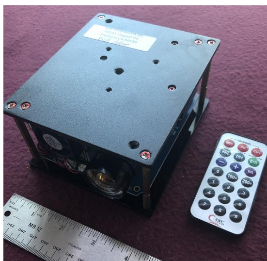
Custom-Built 3-“Color” Blue-Ray LED-DLP Projector
